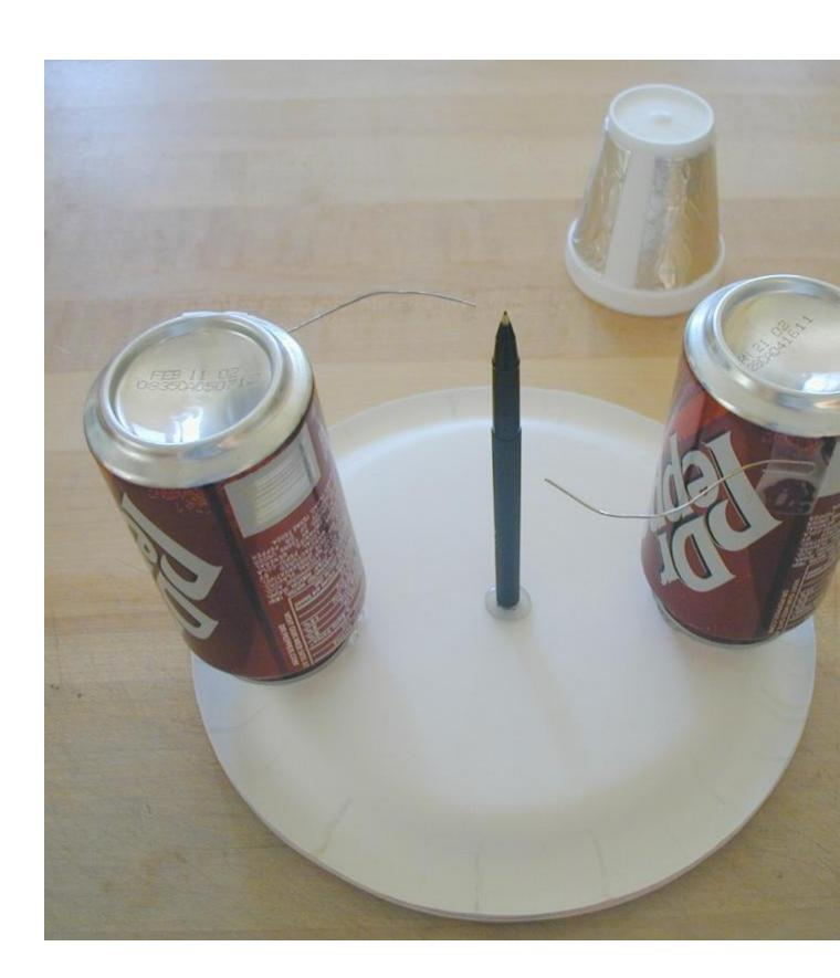
Now put the cup upside-down onto the pen-point. Make sure the dimple fits onto the pen-point. The wires should be about a half inch away from the cup, with the point being closest to the cup. Nothing should be touching the cup except the point of the pen
