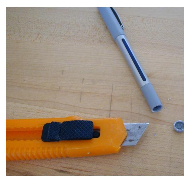
The photo shows the end of the pen, cut off with a sharp knife. The side of the cut end that is facing down has a little dimple that is perfect as a place to accept the point of the other ball-point pen
