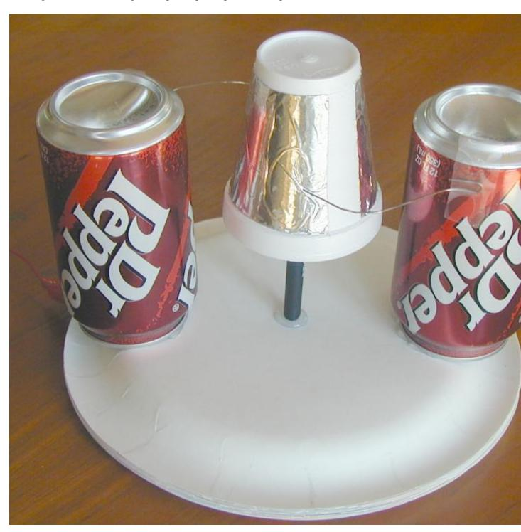
Now connect a wire from the can on the right to a large sheet of aluminum foil pressed against the screen of a TV (or a computer with a CRT screen)
